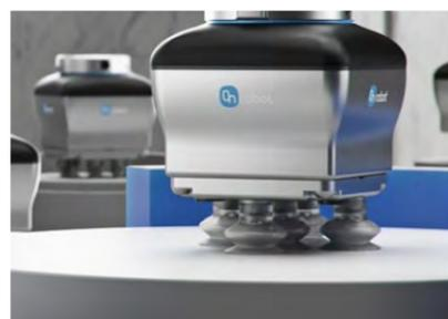
Due to the parcels being stacked on top of each other, and lack of space at the sides of the parcel for a mechanical grip, industry specification suction technologies were studied. Suction is commonplace in industry to move goods, but this has not yet been explored in the drone deliver sector, making it a novel solution.
