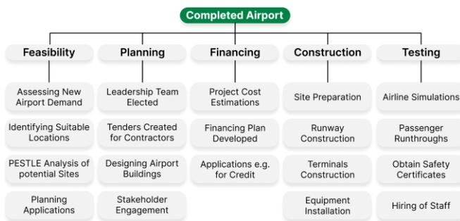
Figure 8 – Partial Project Activity Breakdown [20]
