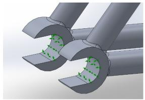
load forces had to use coordinate systems on each of the shells and acted vertically downwards.
