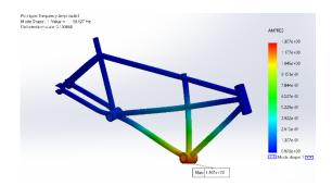
Iterated design with higher resonant frequency.
