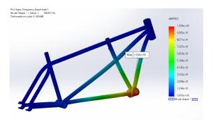
Frequency visual of iterated titanium design
