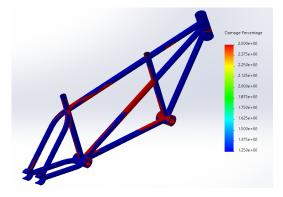
Damage visual of iterated design
