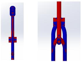
Showing the symmetry of the damage on the frame, and where the higher damage areas are located (red colour)
