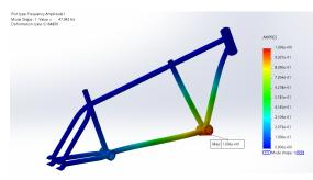
Frequency visual of original design with titanium as the material
