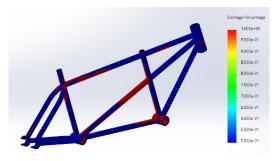
Damage visual of the iterated titanium design.
