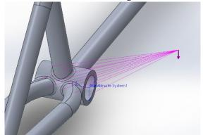
Remote load force was applied to the crankshaft, and the front and rear pedals are in sync with each other due to the chain connecting them on the bike
