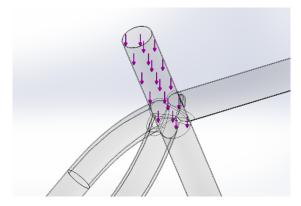
The vertical force is applied 15mm into the tube, which is the length that a seat post is inserted into a bike on average<sup>[6]</sup>
