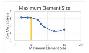
Graph showing that after the maximum element size is less than 5mm, there is
