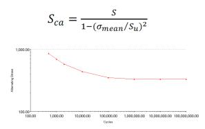
This shows the S-N curve for titanium that had to be manually inputted, along with titanium property values<sup>[7]</sup>
