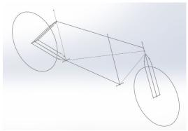
The initial sketch of the frame, using production tandem dimensions<sup>[1]</sup> wheels were included to help visualise and dimension the tubing around them
