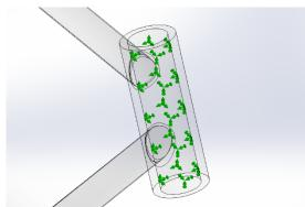
Above image showing the fixed shell, and below showing the rear wheel bearing which can rotate about its axis
