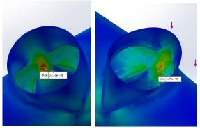
Above showing the before and after effect from mesh control, which helps pinpoint and give a more accurate reading of stress. Below shows where the mesh control was applied to.
