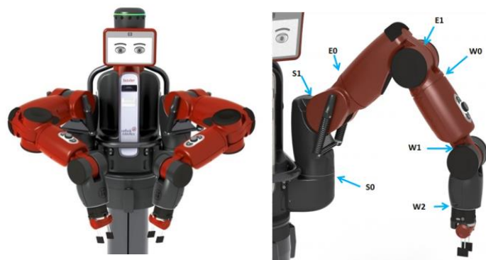
Figure 1: The simplified version of DE NIRO (left), and the locations of its joints (right)
